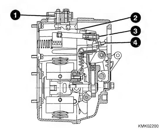
\* Lug cam with torque control
